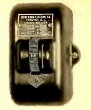
★ Magnetic circuit breakers for protecting tubes and amplifier equipment. Available in models for 50 milliamperes to 35 amps. Time-delay type trips in about 1/100 of a second on short circuit—5 seconds to 8 minutes on 125 per cent load. Instantaneous type may be adjusted for plus or minus 20 per cent of rating. Heinemann Electric Co., Trenton, N. J.— RADIO TODAY.
