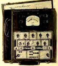
★ Combination tube tester and multi-range meter. Tube tester scale in English and calibrated in micromhos of mutual conductance. Scale length over 4 inches. Reads volts, ohms, mils, mfds., decibels, capacity leakage, and inductance. AC voltmeter accurate on power line and audio frequencies. Housed in walnut case. Model AC-51X. Hickok Electrical Instrument Corp., Cleveland, Ohio.—RADIO TODAX—see also advt. p. 65
