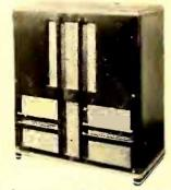
★ Console cabinet loudspeaker for high-fidelity reproduction. Acoustically treated cabinet scientifically coordinated with speaker unit. Power capacity of 10 watts—voice coil impedance 15 ohnis. Substantially uniform frequency response from 60-10,000 cycles. Size 33½ x 28¼ x 16½ inches —finished in black with aluminum trim. List \$133.20. RCA Mfg. Co., Front and Cooper Sts., Camden, N. J. —RADIO TODAY.
